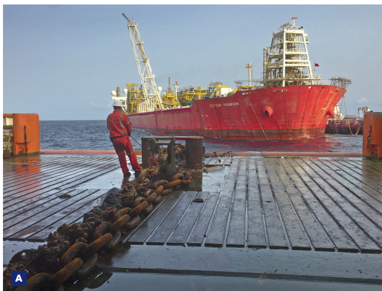
A Mooring chain replacement B Boskalis Heading Control AHT's
